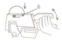
Bend the strip back and feed it through the slot between the white guide pulley (6) and the transport wheel. By operating the grip several times, the label strip is transported inward and tightened. The labeler is now ready for use.
