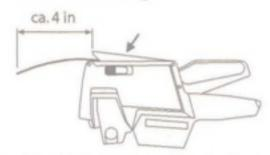
Pull out a strip of labels approximately 4 inches long and close the bottom until it snaps in place.
